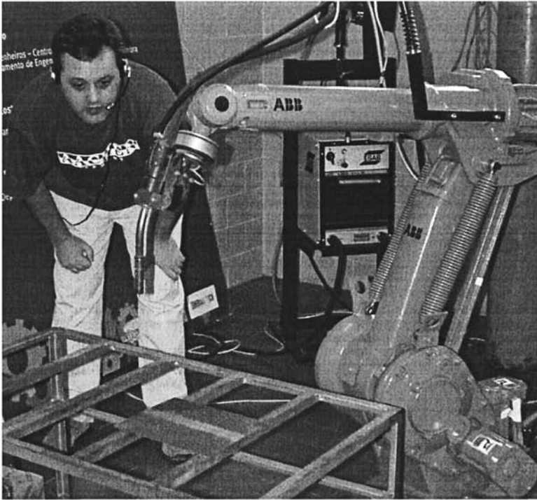
Figure 4.9 Shell of the voice interface application showing the welding operation, and a user (author of this book) commanding the robot using a headset microphone
